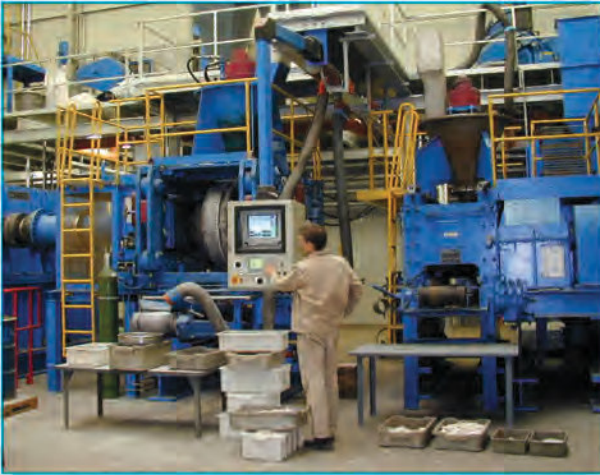
Fig. 5 Köppern pilot plant. Roller press of size 52/10 (left), press 52/6,5 (right)
