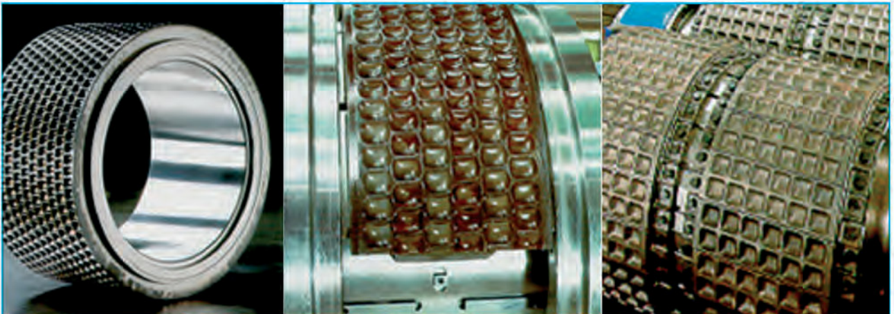
Fig. 4 Various press tools (from left): Tire, segments, strip segments
