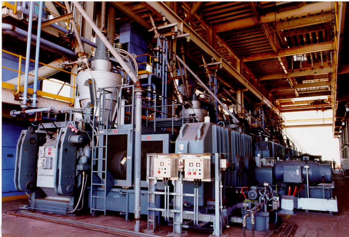
Figure 5: *Briquetting machine for the production of HBI from fine ore.
