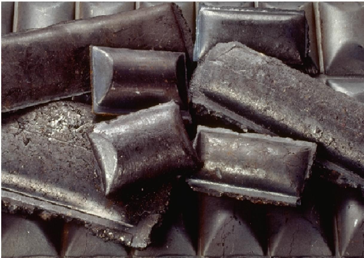
*Figure 2: HBI Briquettes with different shapes and volumes*
