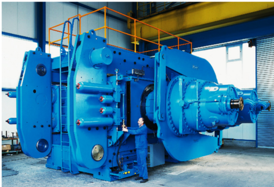
Figure 1 – Picture of a state of the art HPGR by KÖPPER
