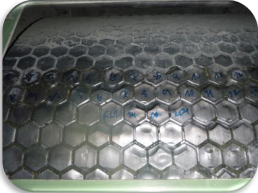
HEXADUR® surface after 53700 hours of operation. The expected lifetime of wear surface is more than 100000 hours of operation.
