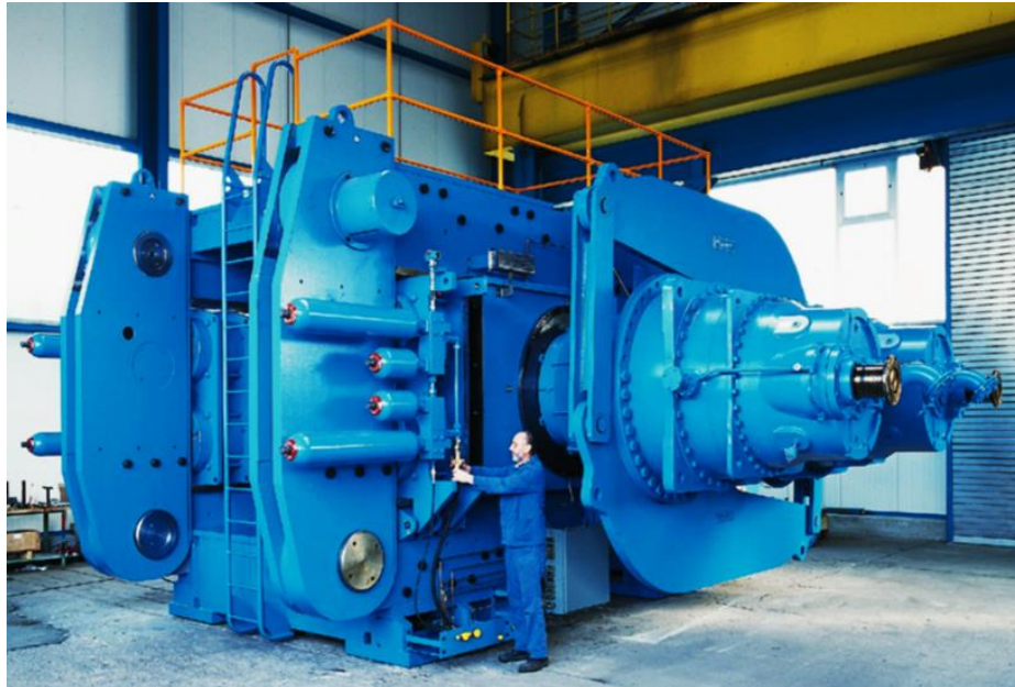
Figure 2 – Typical example of a state of the art HPGR
