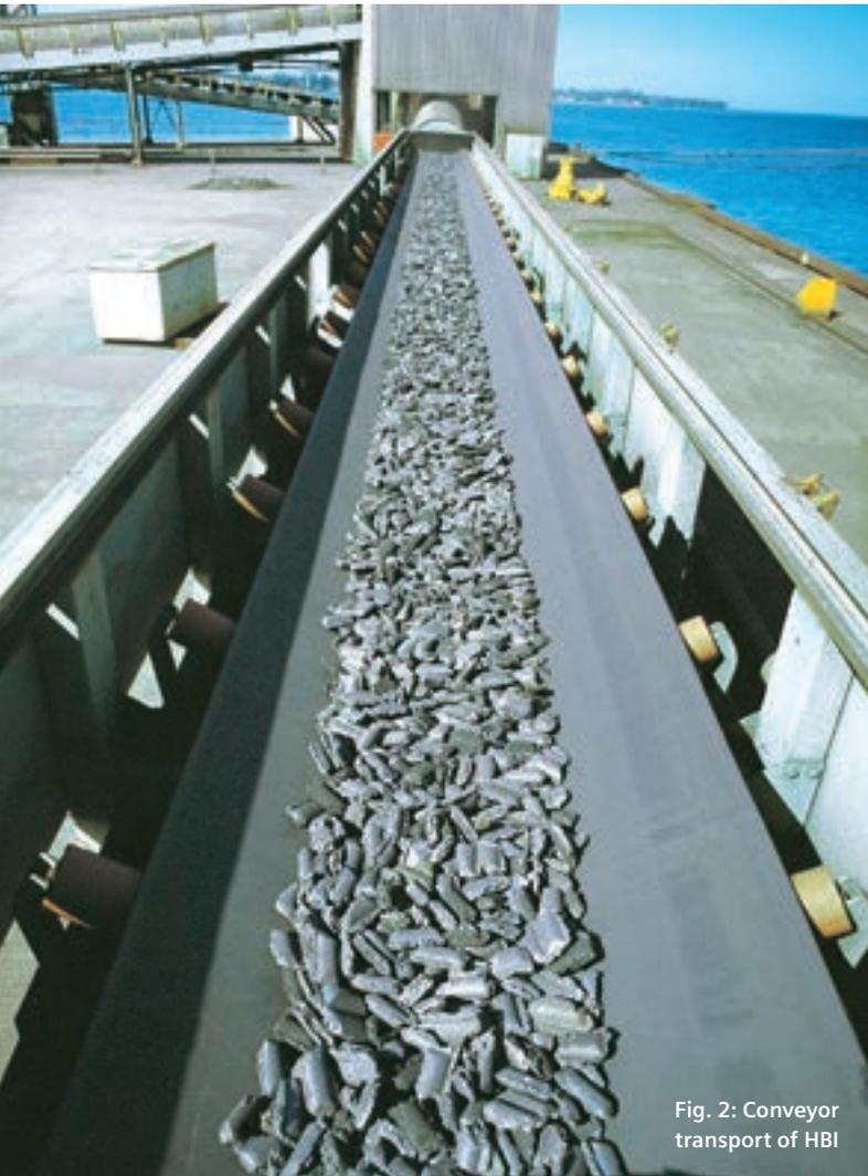
Fig. 2: Conveyor transport of HBI
