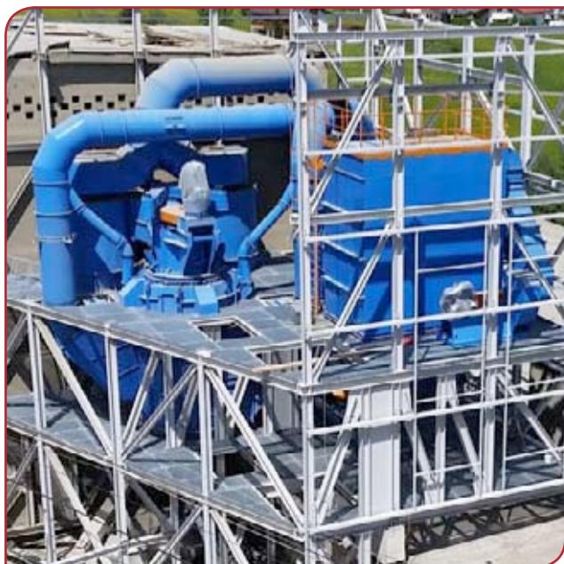
Due to the compact design of the 2-Stage Koesep air classifier and a clear-sighted layout of the new material transport equipment, the upgrade of the grinding plant could be erected while the old system was still in full operation. The integration of the new classifier and the switch-over to the new grinding circuit was then realised with just 40 hours downtime.
