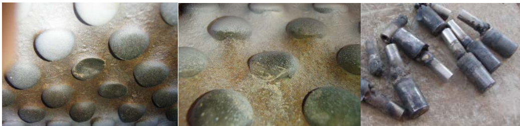
Figure 17 - Examples of broken, chipped center studs and studs removed from wear lining during maintenance (courtesy of Anglo Gold Ashanti).
