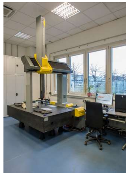
Typ: DEA Scirocco record 10-15-9 Max. workpiece dimension: 1,000 x 1,500x900 mm Accuracy: 2,5 \mu\text{m} + L/300 \mu\text{m}
