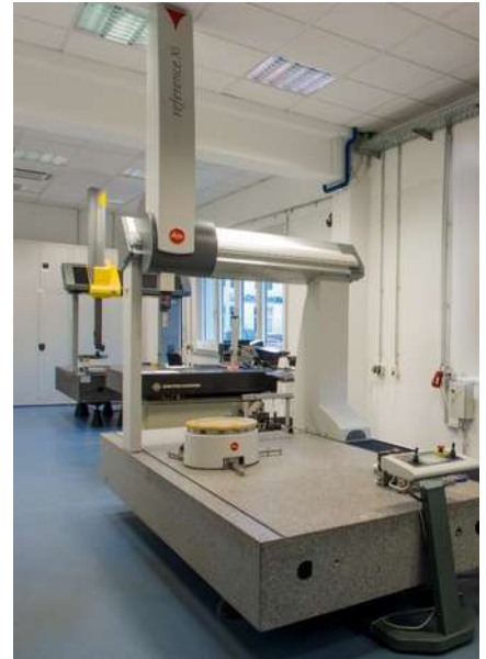
Typ: Referenz Xi 22 12 9 Max. workpiece dimension: 2.200 x 1.200x900 mm Accuracy: 1,8 \mu\text{m} + L/350 \mu\text{m}
