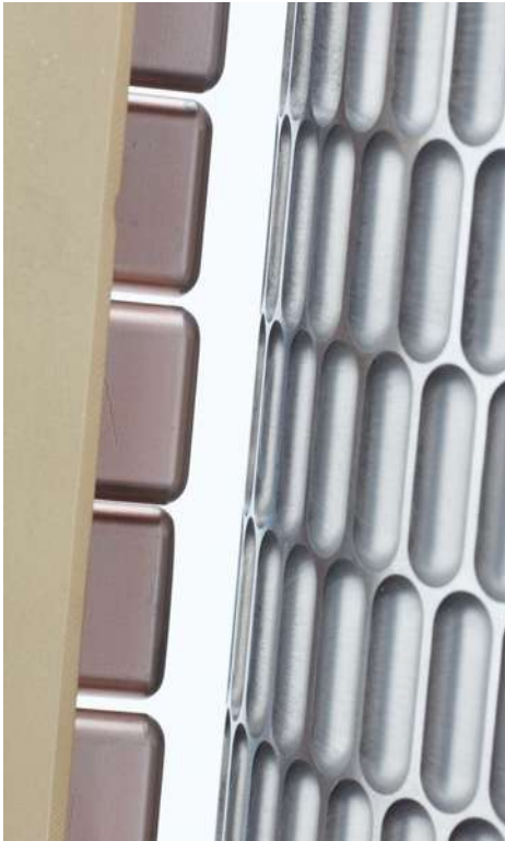
ECM Tool for production of tablets
