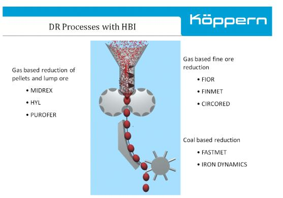
*Figure 12: Direct reduction processes associated with hot briquetting.*
