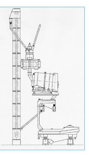
Figure 6: Flowsheet of a briquetting line for hot sponge iron from lump ore and pellets.
